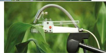
The intensity of the Measuring Light can be sufficiently low for monitoring fluorescence yield without any change in the state of photosynthesis. In addition to the current fluorescence yield ( $F_t$ , in continuous light) and the maximum yield ( $F_m$  or  $F_m'$ , during Saturation Pulses) it is also possible to determine the minimum yield  $F_o$  (after dark-acclimation) or  $F_o'$  (in the illuminated state).
